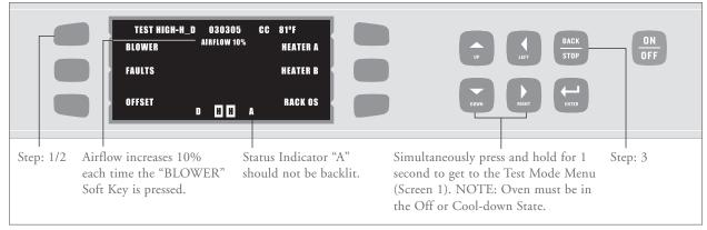
FIGURE 27: Testing the Blower Motor
